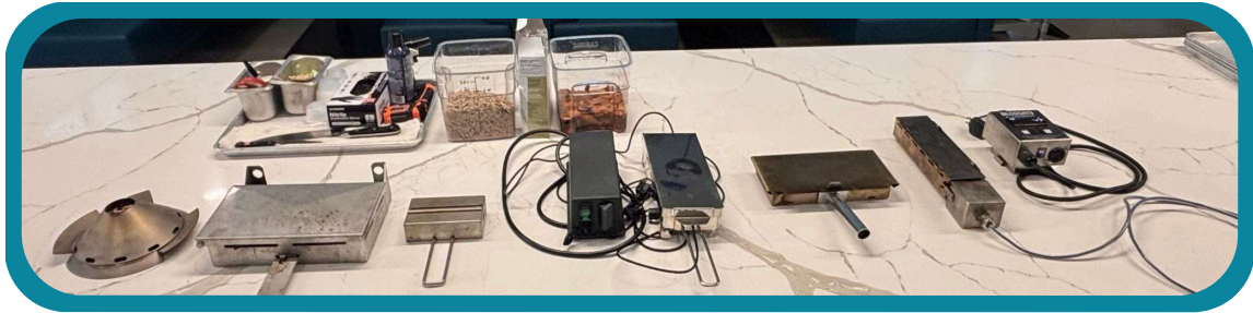
Manufacturer Smoke Kits from left to right: Electrolux, Alto Shaam, Unox, Rational, Convothem, Blodgett
